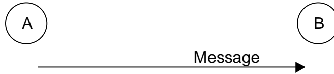
Figure 2 Diagram of a One-Way Message (Asynchronous)
